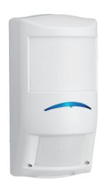
Professional Series TriTech AM Detectors with Anti-mask, LSN are two-wire bus units for commercial and high security indoor applications with the Bosch Local Security Network (LSN). Each detector sends alarm, trouble, tamper, or anti-mask signals through serial communication on the LSN bus. With LSN, there can be a short or open at any point in the loop and all devices still function. The LSN technology supports flexible structures, efficient programming, and high current levels.
